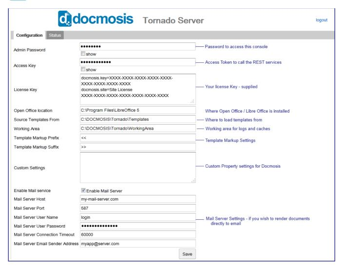
The diagram above illustrates the basics of the areas to be configured. The page provides valuable tool tips for the fields also.
