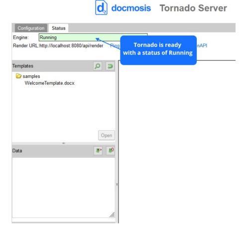
If Tornado has not indicated a running status, examine the log files that will be in your configured Working Area. The logs will provide the diagnostic information about any startup problems.
