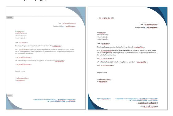
The example template on the left uses the word processor header/footer feature. Whereas the template on the right "simulates" a header/footer, using extended body margins, and placing content in the header/footer positions.
